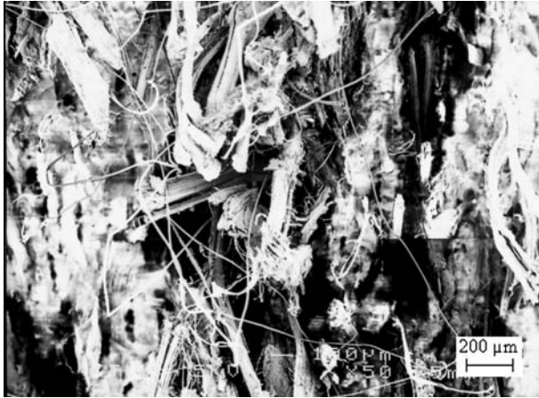
Figure 16 Impact fracture surface of hemp/PF composite (fibre loading 40 vol%).
