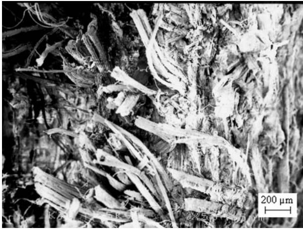
Figure 4 Tensile fracture surface of hemp fibre/PF composite (fibre loading 40 vol%).
